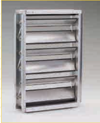
CD 40 — Extruded Aluminum Aerofoil Blades 102mm Max. air leakage – 0.08% Min. size – 152x152mm with single parallel blade and 152x229mm with two blades (opposed or parallel) Max. single section size – 1524x1829mm Max. multiple section size – Unlimited
