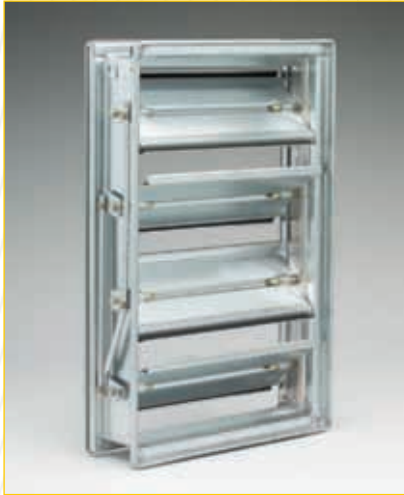
CD35 & CD36 — Galvanized Steel 3V Groove Blades 152mm Max. air leakage – 4.33% without seal and 0.47-1.13% with different type of seals Min. size – 127x127mm with single blade Max. single section size – 1219x1829mm Max. multiple section size – Unlimited
