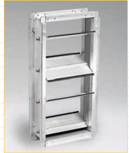
CD51 — Extruded Aluminum Flat Blades 152mm Max. air leakage – 0.16% Min. size – 152x127mm with single blade and 152x229mm with two blades (opposed or parallel) Max. single section size – 1219x1829mm Max. multiple section size – Unlimited
