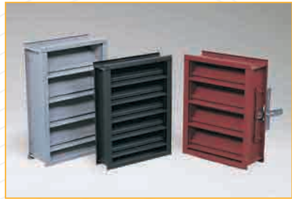
L 375D — High performance Drainable Rain Louvers in Galvanized Steel construction finished in weather-proof paint. Louvers have 102mm depth with 51% free area.
