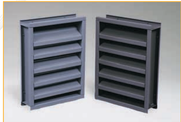
L 330 — Non Drainable Blades in 102mm Deep Frame in Galvanized Steel construction finished in weather-proof paint with 53% free area.
