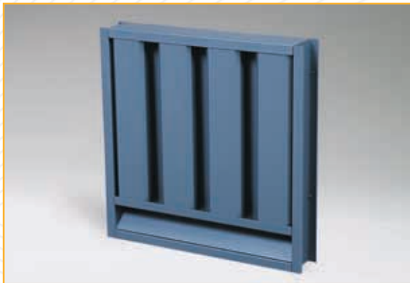
L 5361 — Sand Louvers are designed to remove dust particles in the 140-200 micron size. Made of Galvanized Steel finished in weather-proof paint finish also has low pressure drop and architecturally styled for pleasing appearance. Available in 102mm depth with 25% free area.
