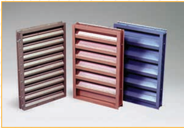
ELF 211D — Thin Line Drainable Louvers in (51mm deep) frame are designed for walls, doors and partitions. These provide attractive appearance with rugged aluminum construction finished in weather-proof paint with 38% free area.
