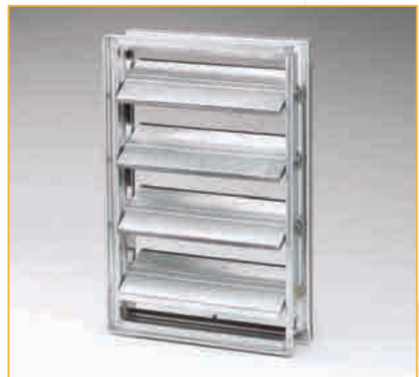
CD 60 — Galvanized Aerofoil Blades 152mm Max. air leakage—0.07%, Min. size—203x254mm Max. single section size—1524x1829m Max. multiple section size—Unlimited
